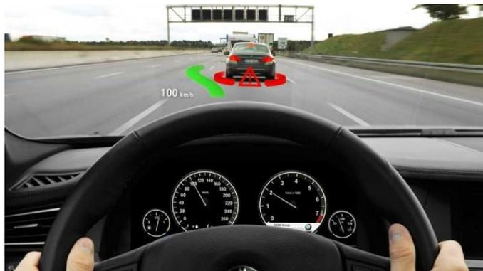
Figure 3. BMWs new heads-up displays project virtual information of the cars windshield
